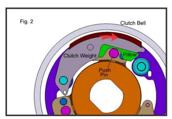
bell to proceed the initial slippery clutch-in. The clutch weight is slippily contacting with the bell but the push pin is unactuated yet (Fig.3).
